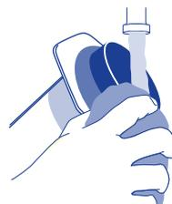
Always store the **AeroPress** with the plunger pushed all the way in, or completely removed, to avoid compressing the seal.
